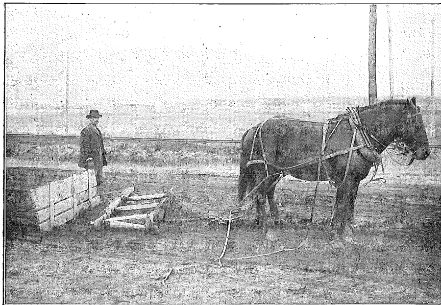
FIG. 13. — The split log type of drag after the "King" design, showing removable platform.
